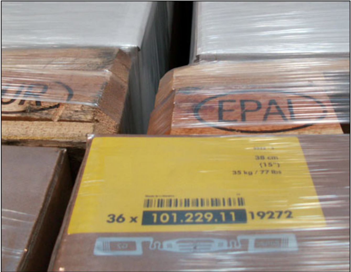
When a pallet is loaded with boxes of lamps, an RFID label is attached to one of the boxes.
