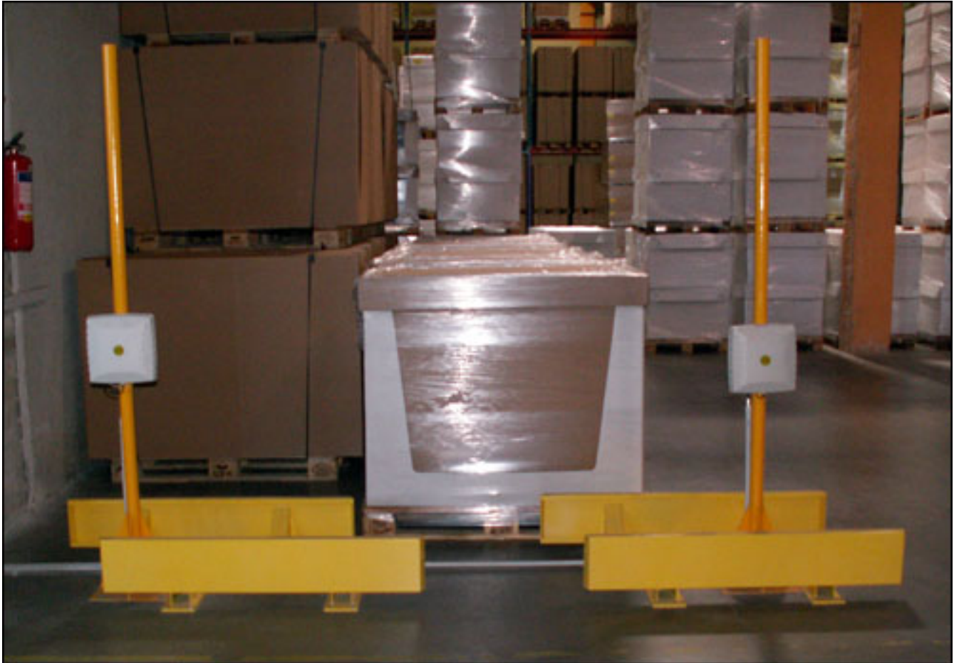
As a pallet loaded with boxes of lamps is taken to the warehouse, it passes an RFID portal, which reads the tag attached to one of the boxes, thereby recording that it has been moved into storage.
